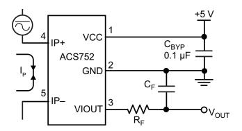
Application 1. The ACS752 outputs an analog signal,  $V_{OUT}$ . that varies linearly with the uni- or bi-directional AC or DC primary sensed current,  $I_P$ , within the range specified.  $C_F$  is recommended for noise management, with values that depend on the application.
